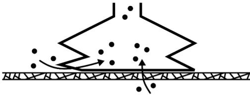
Leaking workpieces can be even harder to identify. Things that look completely tight might not be tight at all. A typical example is coarse cardboard boxes. The thin outer layer is often requiring a lot of air flow to create a pressure difference over it (see figure below).
