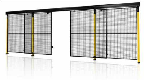
Double sliding without rail, has an opening of 6 meters and no upper limitation. The door is perfect when handling large volumes carried by overhead crane or forklift. Maximum width 2 x 3000 mm and maximum height 2300 mm.
