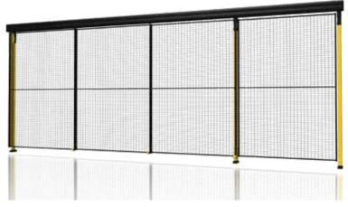
Single sliding door without rail. An ideal solution for an opening with no overhead obstruction and where the need for a large opening isn't necessary. Maximum widths 900 mm and 1400 mm, maximum height 2300 mm.
